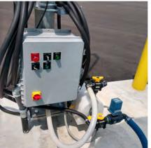
GVM's Overhead Spray Systems (OSS) are multifunction liquid deicer dispensing systems designed to pre-wet truck loads of solid de-icing materials. Pedestal Pre-Wet Systems allow users to pre-wet multiple truckloads with only one dispensing system. Pedestal systems are also capable of loading and unloading truckmounted pre-wet tanks, returning the de-icing liquids to bulk storage tanks, and draining tanks for end-of-season maintenance.
